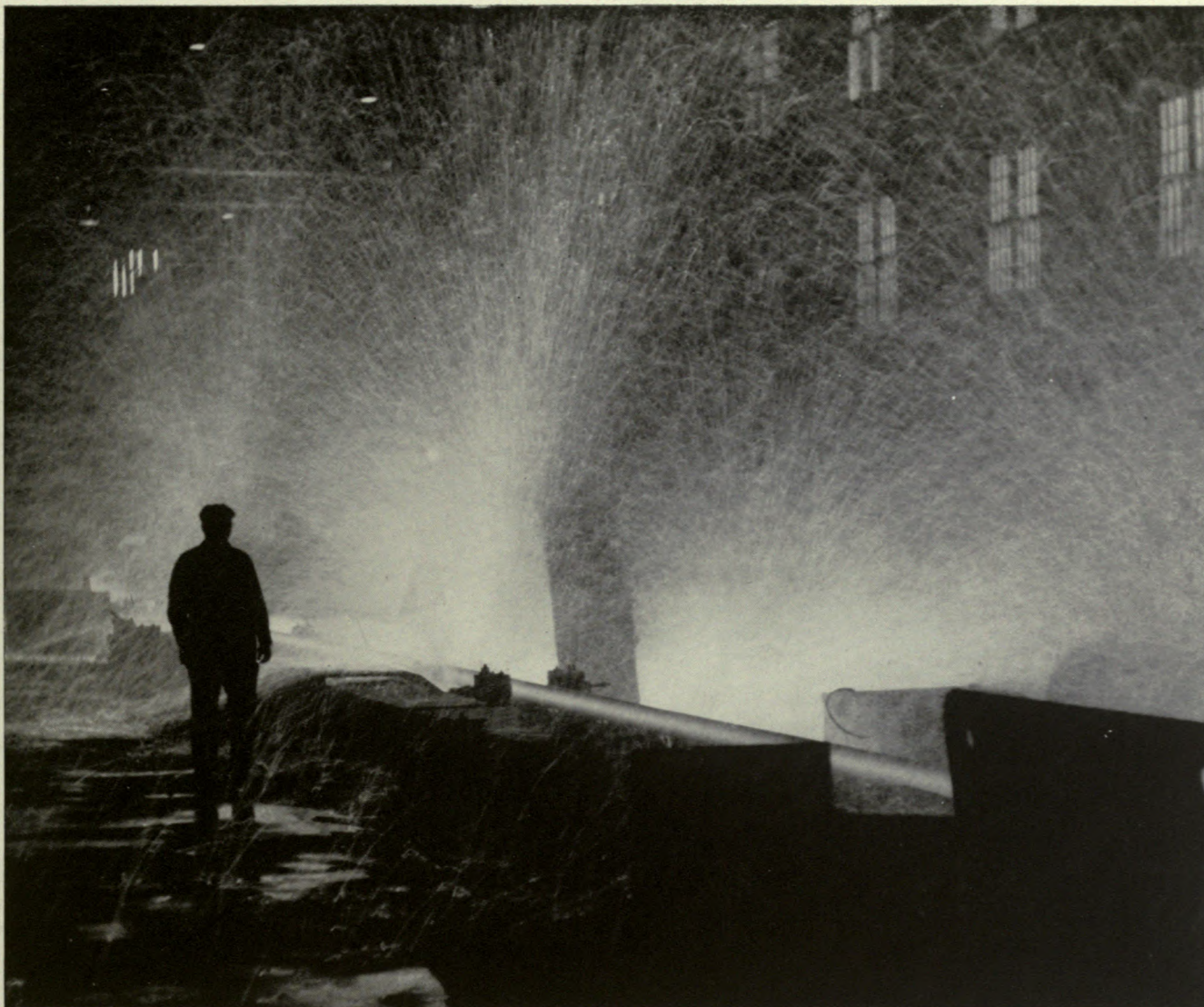
A shower of sparks fly in a U. S. Steel rail mill as saws cut a long rail into suitable lengths for the railroads.
